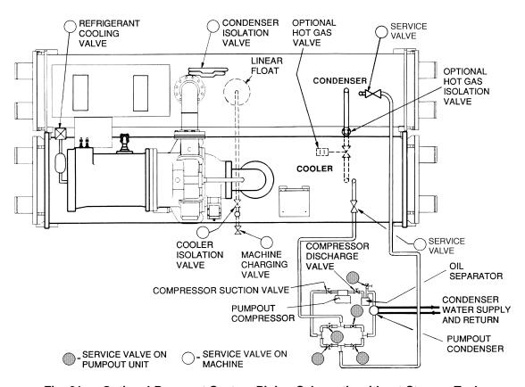
Fig. 21 — Optional Pumpout System Piping Schematic without Storage Tank
